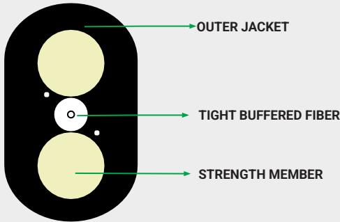
STL RapidDrop Flat Drop Dielectric Fiber Optic Cable offers ease of installation in an easy access, single-buffer design. This is a Central inner subunit of cable is made up of single optical Fiber with buffer presented and is enclosed in a thermoplastic sheath. The cables have two embedded strength members for anti-buckling property. The dielectric version eliminates any bonding and grounding requirements.
