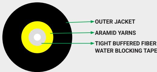
\* Typical Construction Diagram - Not to Scale
