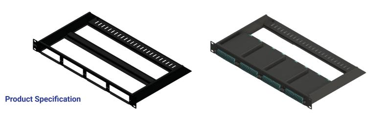
STL 1RU panel is a custom designed panel for MPO Cassettes. Made of CRCA steel sheet with black powder coating, is very sturdy and provides long service life. Flat 1RU panel with 19 inch width is best suited for mounting inside the equipment racks. The rear cable support bar with slots for Velcro tie is the ideal solution to support and secure the connecting cable loop without any entangle with other adjacent cables.
