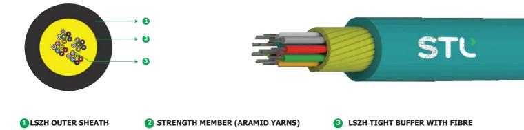
\* Typical Construction Diagram - Not to Scale
