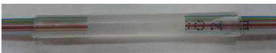
Figure 15- Spliced ribbon fiber with protection sleeve
