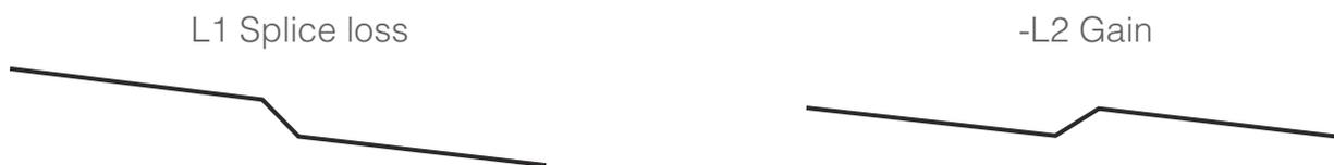
Fig. 16: OTDR trace at splice point
