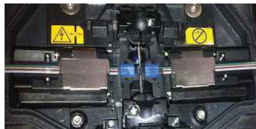
Figure 12- Splicer unit with ribbon holders
