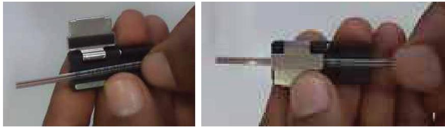
**Figure 5- Placing of Fiber Ribbon in holders**
