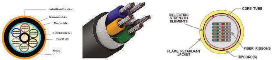
Figure 1- Cross Section: Generic Indoor Ribbon Backbone Distribution Cable
