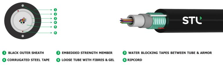
\* Typical Construction Diagram - Not to Scale
