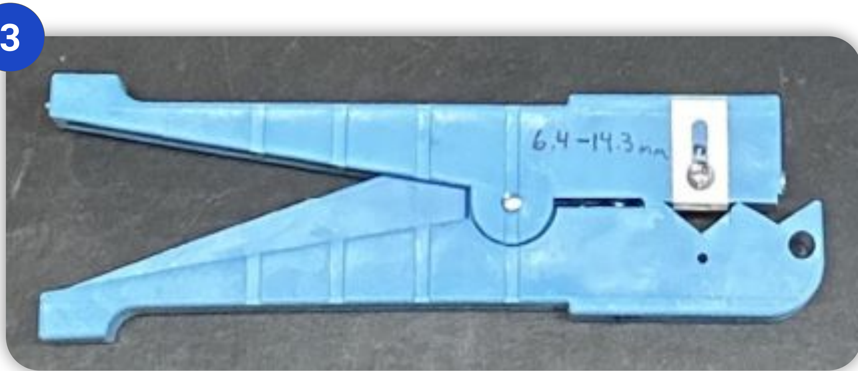
Tool Name: Ideal Buffer Tube Stripper 45-164 (6.4 – 14.3 mm)
