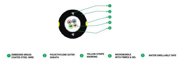
\* Typical Construction Diagram - Not to Scale
