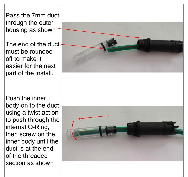
Note: When installing the DP Overhead a micro-duct/cable coil must be provided to enable the DP to be brought to the ground for maintenance work. For the Maintnence Coil use 5/3.5 UV Stable Micro-Duct and UV Stable Reducers to convert from 7mm to 5mm Micro-Duct.
