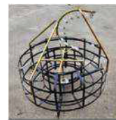
Intermediate Cable Storage Device (GMP)
