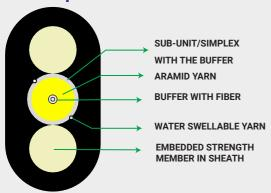
\* Typical Construction Diagram - Not to Scale
