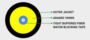
The construction of OptoPull with 3mm round drop cable features an FR TPU sheath, ensuring it meets higher fire safety requirements. It is equipped with an easily removable, rugged thermoplastic jacket that offers UV protection. The cable is flexible, lightweight, and easy to handle and install, making it highly user-friendly. Additionally, the 850  $\pm$  50  $\mu m$  tight-buffered fibers support fast field installations, enhancing its practicality for various applications.
