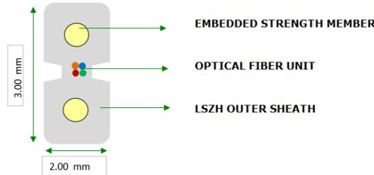
\* Typical Construction Diagram - Not to Scale
