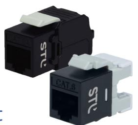
Category 6 and 6A UTP RJ45 Keystone jacks conforms to class E and  $E_A$  performance respectively, due to their small form design, they are perfect for compact and sleek applications. Each jack is available with a 90° and 180° termination design, wiring diagram, and conductor protection cap.
