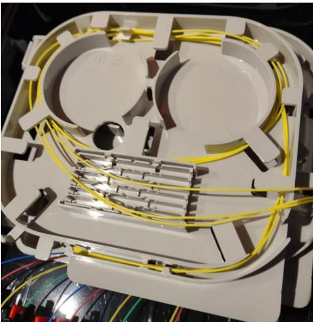
Re-route the splitter inputs from the base to the top tray as shown. Then run the network inputs to the top tray as shown in the network installation guide and splice.
