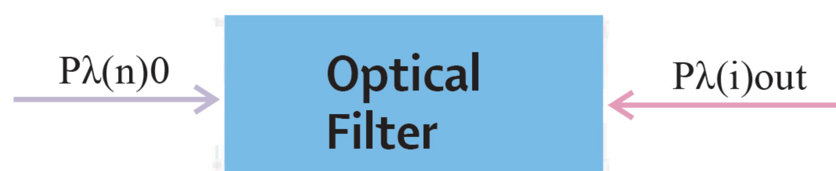
Figure18 – Block Diagram of Optical Filter Breaking Out Wavelength “i” From a Signal Containing “n” Wavelengths
