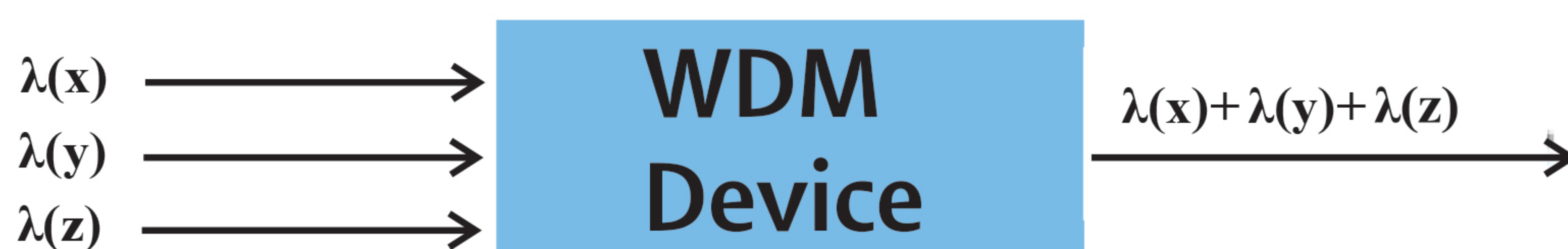
Figure16 – Schematic Drawing of WDM Device Combining Three Wavelengths From Separate Fibres into Three Wavelengths on One Fibre.
