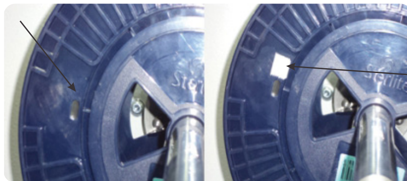
Figure 8: Cutting and fastening fiber inner end on spool flange
