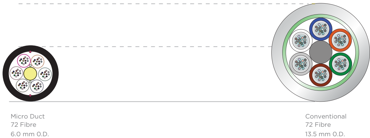
Figure 5- Comparison of STL's Micro-Duct Optical Cable to a 72 Fibre Conventional Optical Cable
