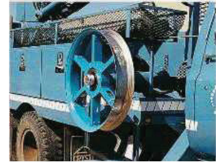
Side take-off winch with slip clutch (Condux)
