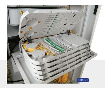
Where full and easy access at both sides of the connection is required, sliding trays are used instead of front patching, pivoting ones. A connector can be patched in a different position within the same tray with a perfect control of the extra length.
