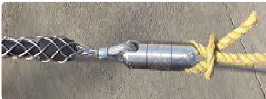
Figure 4 - Anti-twist device/ swivel placed in between cable end and pulling rope
