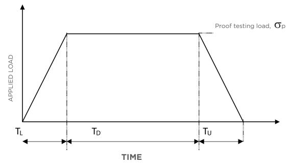
where,  $T_L$  is the loading time (time to reach zero to proof testing load)  $T_D$  is the time of applied proof testing load (also known as dwell time)  $T_U$  is the unloaded time (time to come to zero load level)
