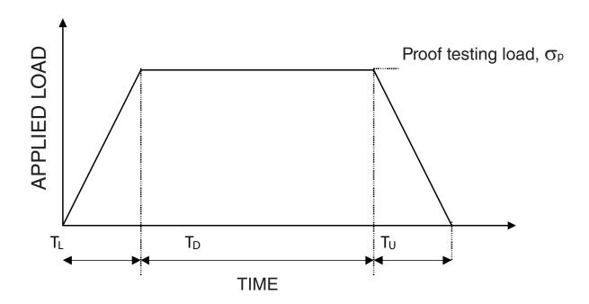
where,  $T_L$  is the loading time (time to reach zero to proof testing load)  $T_D$  is the time of applied proof testing load (also known as dwell time)  $T_D$  is the unloaded time (time to come to zero load level)
