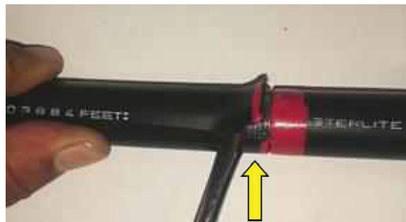
Figure 5- Cable jacket access for removing/take off
