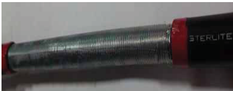
Figure 8- 15 cm window cut without outer sheath
