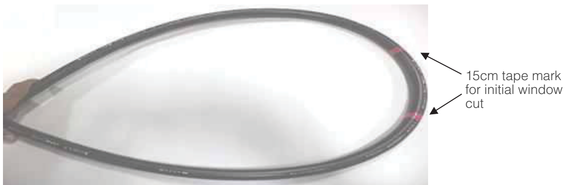
Figure 1- Cable layout for mid-span access
