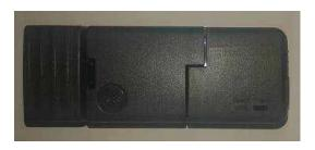
Figure 6- Hot jacket stripper/ thermal stripper
