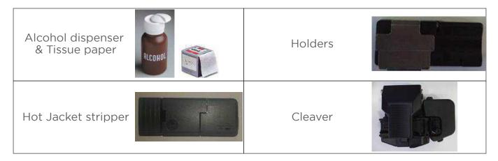
Figure 1- Common Tools and Materials for Fusion Splicing
