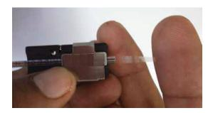
Figure 9a- Cleaning of stripped fiber
