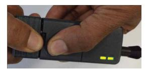
Figure 8b- Hot jacket stripper/ thermal stripper operations
