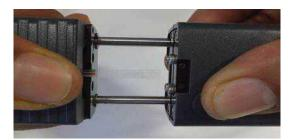
Figure 7- Placing the holder in Hot jacket stripper/thermal stripper
