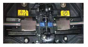
Figure 12- Splicer unit with ribbon holders
