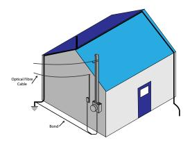
Equipment and building protection is provided by low impedance grounding and bonding between electrical services, protective devices, equipment and other conductive objectsso that faults or lightning currents do not result in hazardous voltages within the building. Also, the proper operation of over current protective devices is frequently dependent upon low impedance fault current paths.
