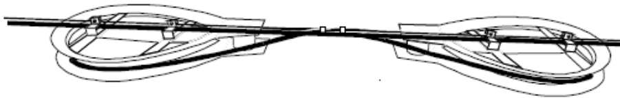
Figure 6- Pair of Snow Shoes Used to Store Slack Cable at end of each Cable End
