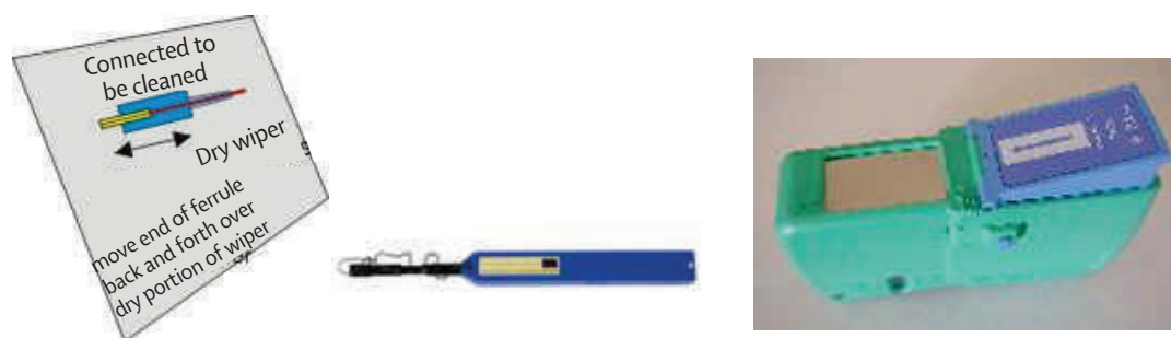
Figure 11 – Dry Wipe Process Illustration (Using Dry Wipe, Tool, or Cassette)
