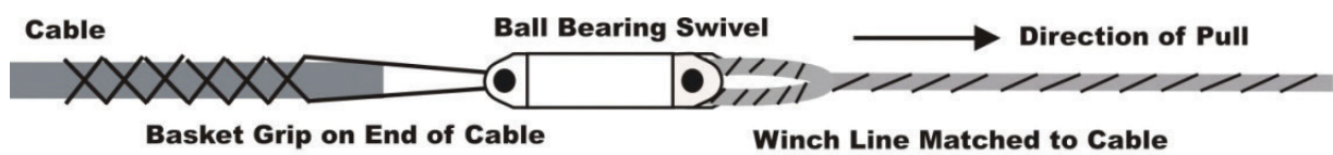
Figure 10 - Cable placement array using ball-bearing swivel to connect winch line to cable
