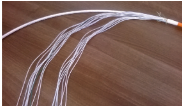
Figure 28 Unwind the loose buffer tubes in the cable core from around the CSM.
