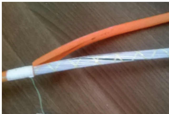
Figure 9 Longitudinal slit in cable sheath is made with the rip cord(s).
