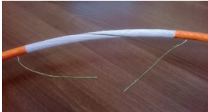
Figure 23 15 cm mid-span access window is exposed to cable core with rip-cords after the jacket has been removed.
