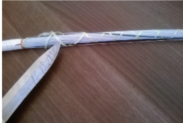
Figure 25 Cutting the binder yarns.
