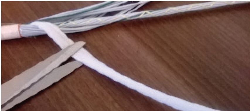
Figure 12 Cut the water blocking tape (in case of 288F microcable design).
