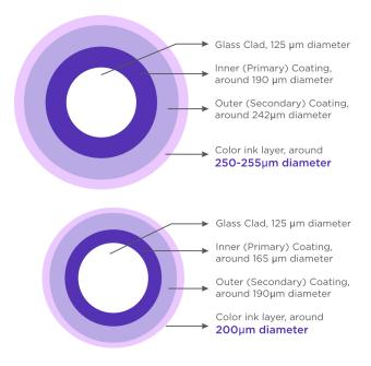
Figure 1: Schematic Cross sectional view of SMF (not to scale)
