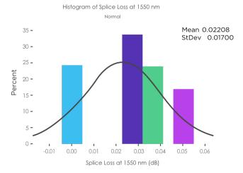
Figure 4: Splice loss between 200 micron and conventional SMF at 1550 nm
