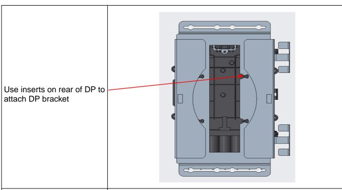
For single pole mount, fix pole bracket as shown using screws top and bottom.
