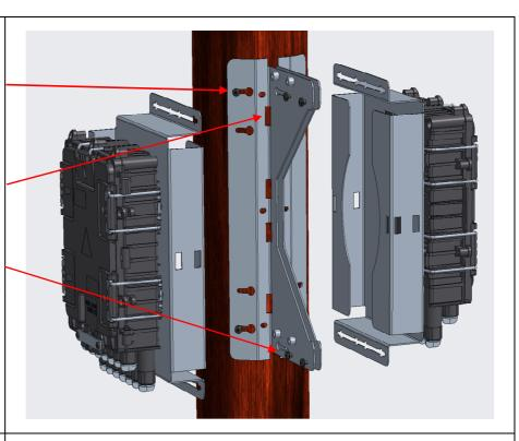
Image showing double pole mounting.
