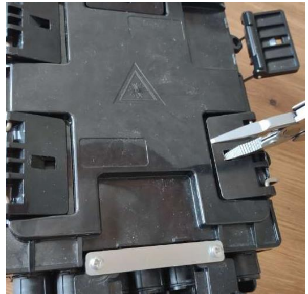
Using a pair of Pliers or a Screwdriver open the 5 spring latches
