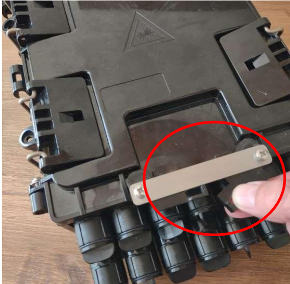
To open the DP, slide the 2 tabs down at the bottom of the lid.
