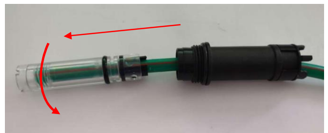
Push the inner body on to the duct using a twist action to push through the internal O-Ring, then screw on the inner body until the duct is at the end of the threaded section as shown.
