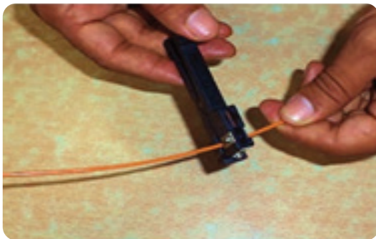
Traditional Fibre Cable Tube Stripped by Tool
