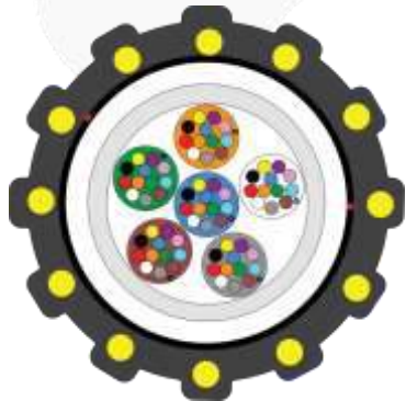
Micro Ribbon Cable 432F (12F Ribbon x 36)
