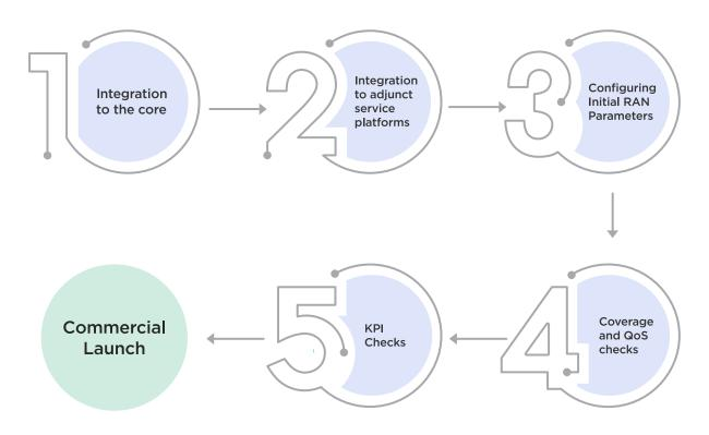
Figure 5 - High level process of new site/RF Carrier launch
