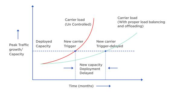
Figure 6 - Automation to improve traffic handling efficiency delays the need for new RAN capacity
