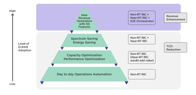
Figure 4 - RIC use cases: A high level classification and calibration with O-RAN adoption
