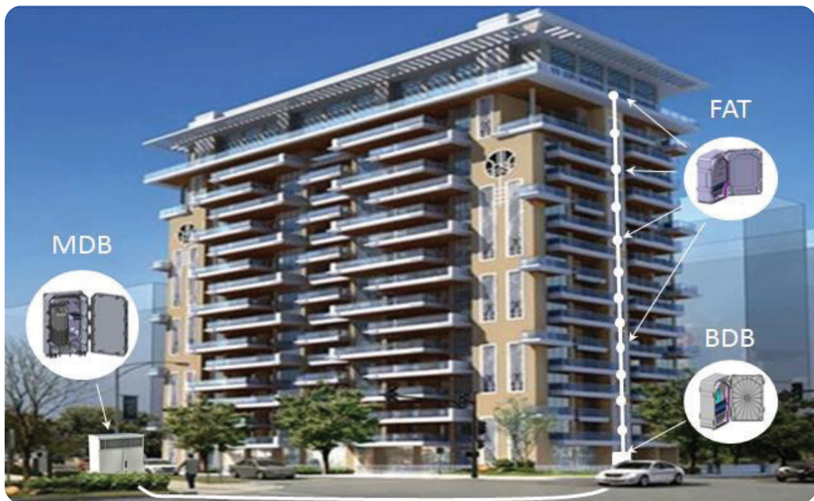
Figure 4 Typical MDU deployment scenario of Sterlite Tech's Plug & Play FTTH solution
