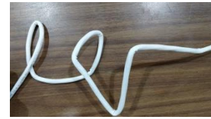
Figure-09 : Cable bent too much
