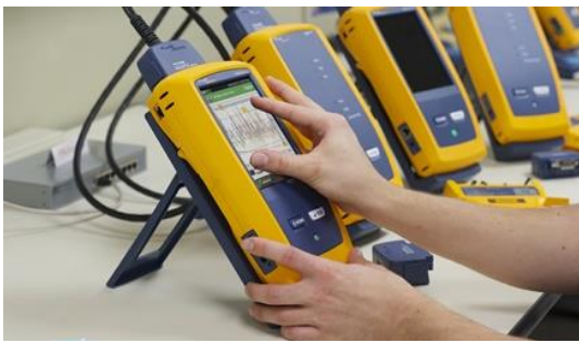
Figure-02 : DSX-5000 Network Analyzer
