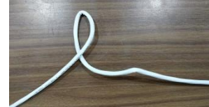
Figure-08 : Cable bent slightly
