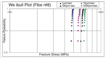
Fig.3 Weibull plot of two-point bend strength values at four extension rates of Fiber# 1,4,5 & 8
