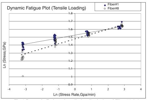
Fig.1 Dynamic Fatigue (tensile loading) plot of Fiber#1 & 8
