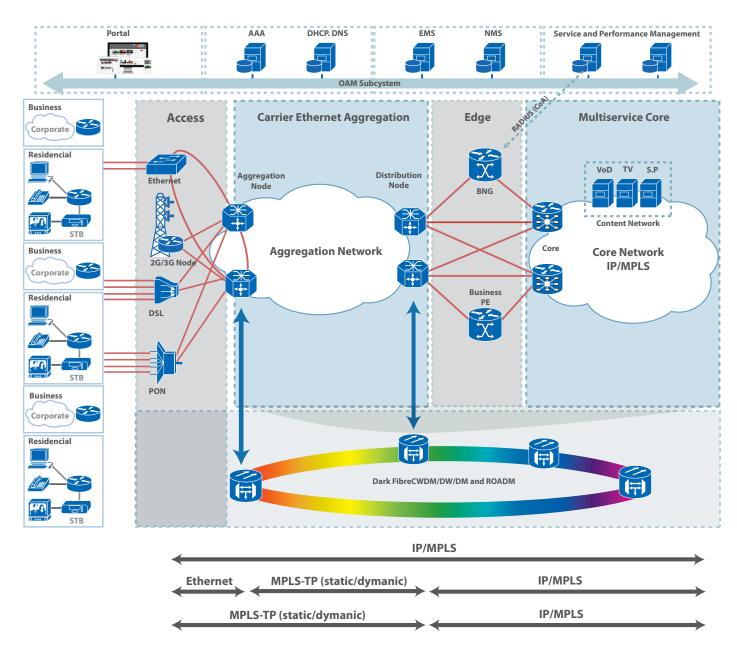
fundamental idea is that dedicated OAM packets are interspersed into the associated user traffic flows. These OAM packets are created and processed by maintenance end point. Maintenance intermediate points can also process these OAM packets and may collect data or raise alarms. The tools can be categorised in proactive OAM functions that are running all the time and on-demand monitoring functions.
