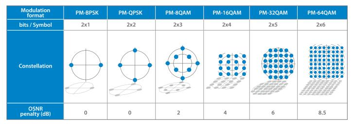
Figure 4: Comparison of modulation techniques for 100G and beyond
