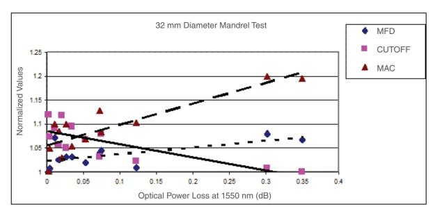
Fig. 5 : Plot of optical power loss at 1550 nm with MFD, Cut-off and MAC value for 32 mm diameter mandrel test
