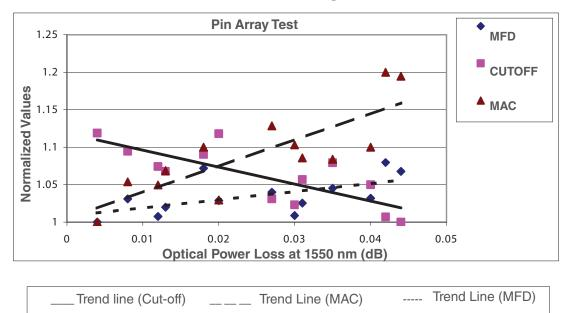
Fig. 4 : Plot of optical power loss at 1550 nm with MFD, Cut-off and MAC value for Pin Array Test
