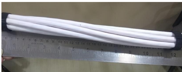
Figure – 10 Alien Crosstalk Bunch with No gap
