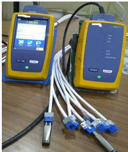
Figure 7 – Alien Crosstalk Measurement with Field Analyzer
