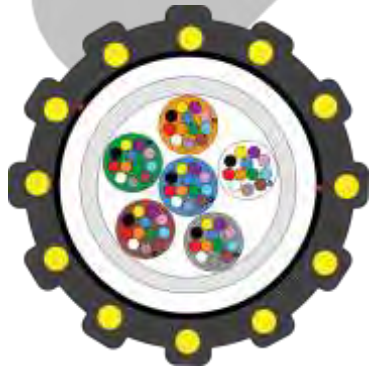
Micro Ribbon Cable 432F (12F Ribbon x 36)
