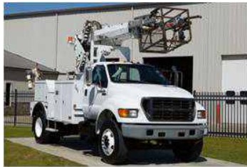
Cable Placing Truck (Canada)
