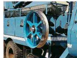
Side take-off winch with slip clutch (Condux)
