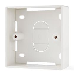
STL high quality gang box/back box are the best suited accessory for placing the faceplates on the plain surface. Made with high quality ABS material complied to UL 94V-0. With the dimension of 86mmX86mm is a perfect fit for the STL British style face plates with single and dual ports. Gang box /back box is provisioned for the back side cable entry ensure the proper alignment of cable with the Keystone Jacks.
